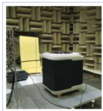
Research on noise optimization in the anechoic chamber of the University of Sherbrooke
